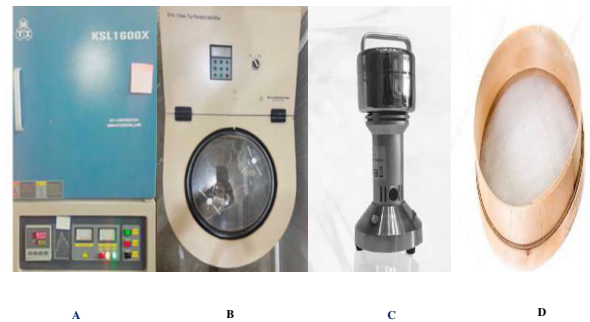
Figure-3. Shows the apparatus used to make H.A.P powder from Eggshells: (a) Furnace; (b) Planetary ball; (c) steel kitchen mill; (d) Sieve.
