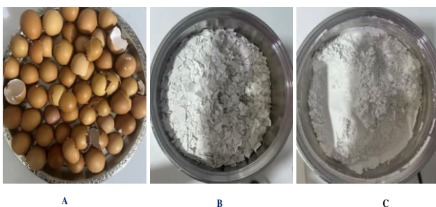
Figure-2. Depicts the process of producing HAP powder from eggshells. Egg shells were cleaned in A, broken and calcined in B, and crushed and milled in C.
