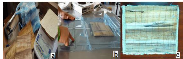
Figure 2. The manufacturing process of the Banana/sisal/bioepoxy composite. a) Determination of the weight in the reinforcement, b) mould for infusion and c) laminate obtained.
