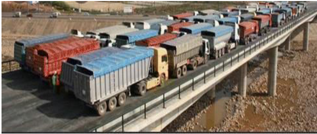
Figure-2. Static load test on the bridge [55].
