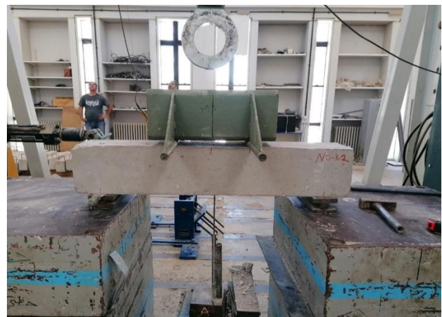
Figure-4. Four-point load test.
