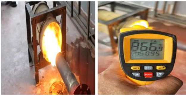
Figure-2. Process of burning marble waste powder.
