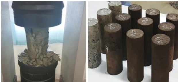
Figure-11. The compressive test process for DCT, DCL, WCT and WCL types of concrete samples.
