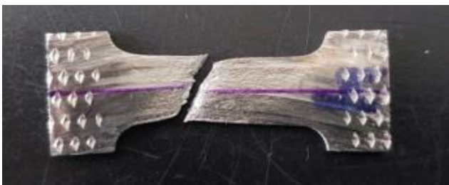
Figure-12. Failure for specimen two after tension test. Source: Authors.
