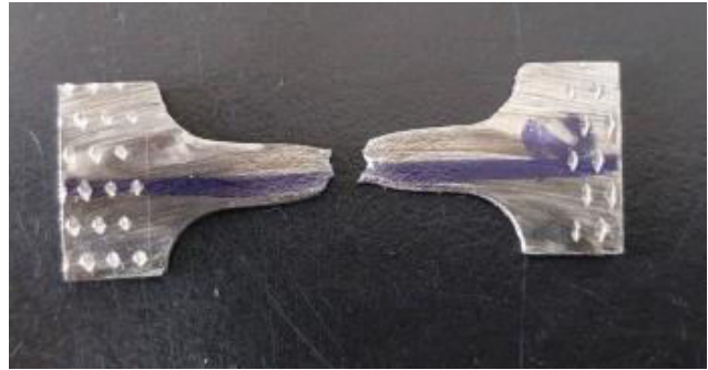
Figure-8. Failure for specimen 2 after tension test. Source: Authors.
