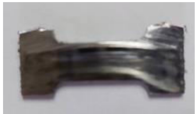
Figure-4. Thickness 1 mm probe cut. Source: Authors
