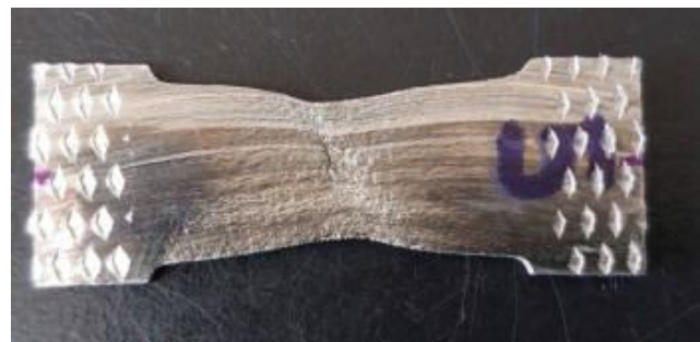
Figure-14. Failure for specimen two after tension test. Source: Authors.
