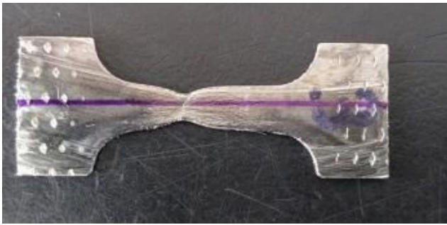
Figure-10. Failure for specimen 2 after tension test. Source: Authors.
