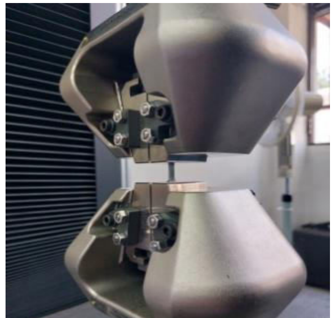
Figure-5. Tensile test of the specimens in the machine.
