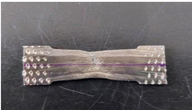
Figure-6. Failure for specimen 1 after tension test. Source: Authors.
