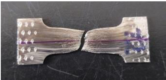
Figure 16. Failure for specimen 12 after tension test. Source: Authors.
