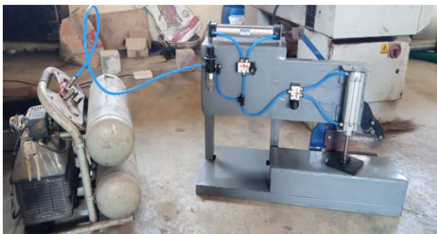
Figure-5. Pneumatic sheet metal clamping and shearing machine setup.
