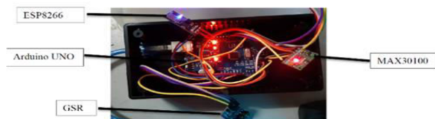
Figure-3. The laboratory prototype of the developed system.
