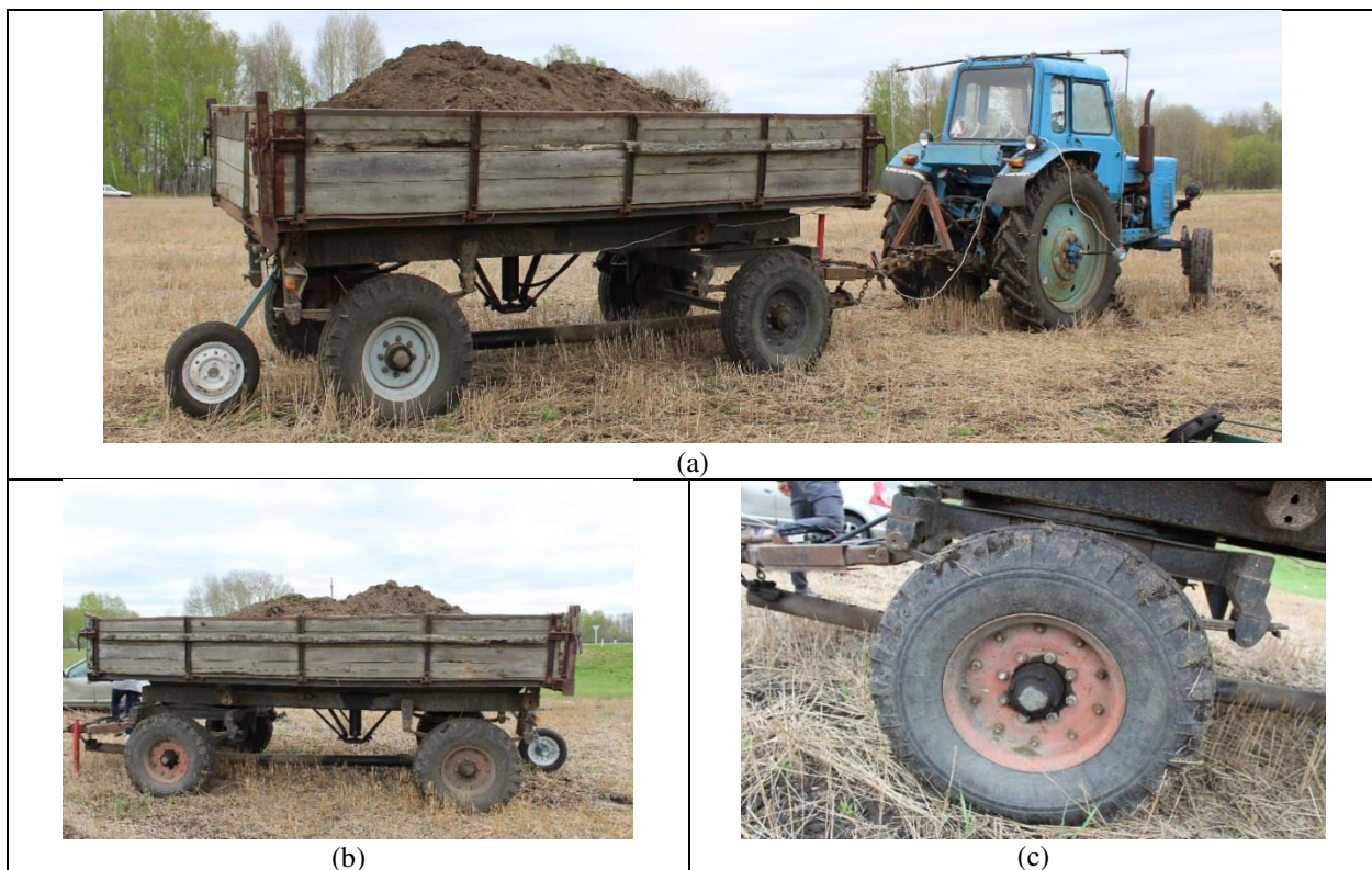
Figure-1. Tractor transport aggregate MTZ-80 + 2PTS-4M: a - general view of the aggregate; b - tractor agricultural trailer 2PTS-4M; c - trailer running gear with tires Voltyre Ya-324A (9.00-16).
