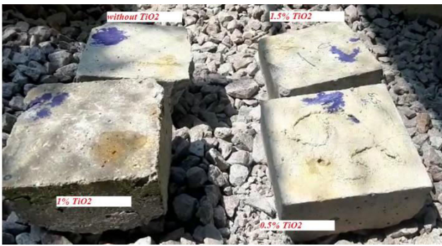
Figure-10. Methyl orange test on CC and SCC after 6 hours.
