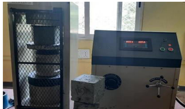
Figure-4. Compressive test on SCC.
