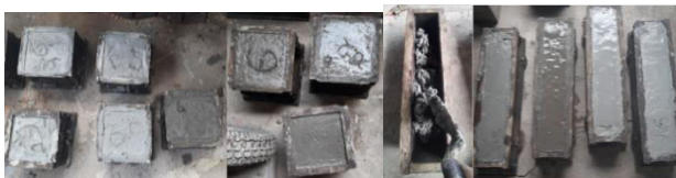
Figure-2. Casting of self-cleaning concrete.
