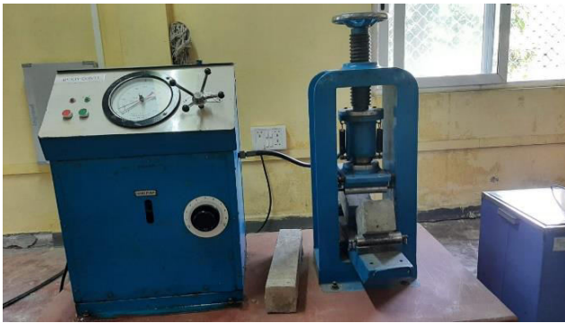
Figure-6. Flexural strength test on SCC.
