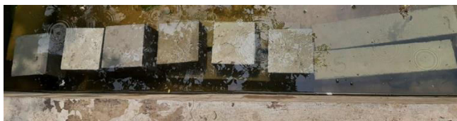
Figure-3. Curing of self-cleaning concrete.
