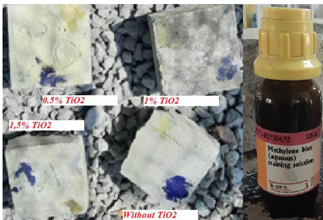
Figure-11. The reduction in methylene blue on CC and SCC.
