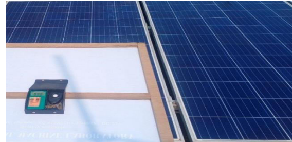
Figure-24. Single PV panel partially shaded
