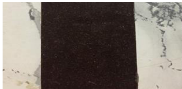
Figure-3. Coconut shell-reinforced polymer composite plate.
