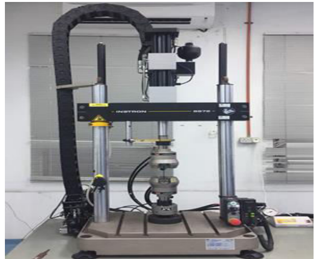
Figure-5. Universal Tensile Testing Machine with a load capacity of 25 kN.
