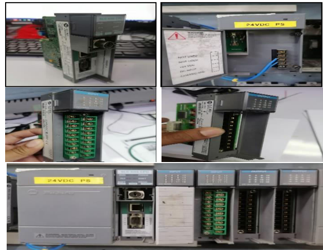
Figure-7. Hardware Designing of Allen – Bradley Programmable Logic Controller.
