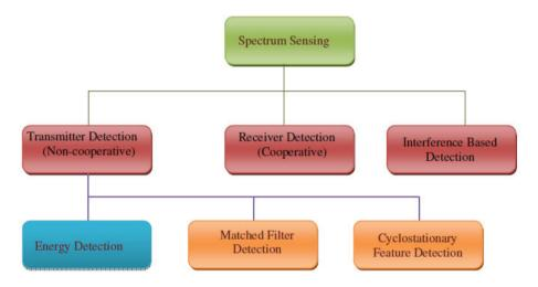
Figure-2. Spectrum detection techniques.
