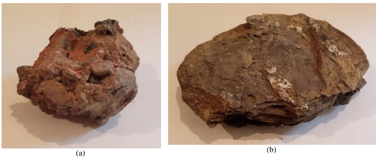
Figure-3. General view of the rock waste: A - burnt mass; and B - slightly burnt mass.
