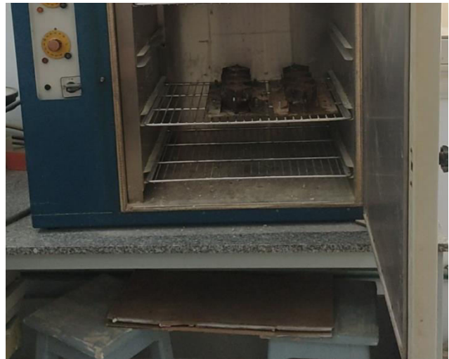
Figure-6. Heating NLGP cubes.
