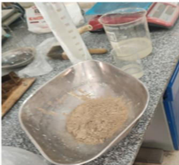
Figure-3. Fly ash ready to be mixed.
