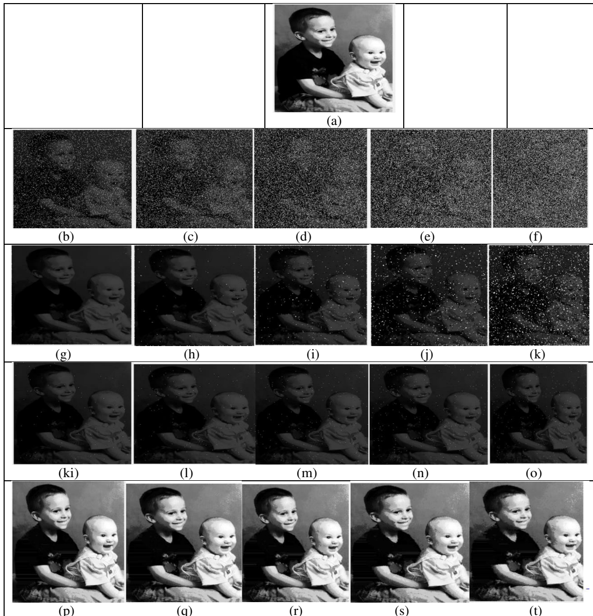
Figure-2. Removal of Salt And Pepper Noise of Sample B (a) Original image (b) Corrupted Image With 10% Noise (c) 20% Noise (d)30% Noise (e)40% Noise (f)50% Noise (g- k)Restored of Image using SMF for Different noise respectively (ki-o) Restored of Image using AMF for Different noise respectively (p-t) Restored of Image using MMF for Different noise respectively.
