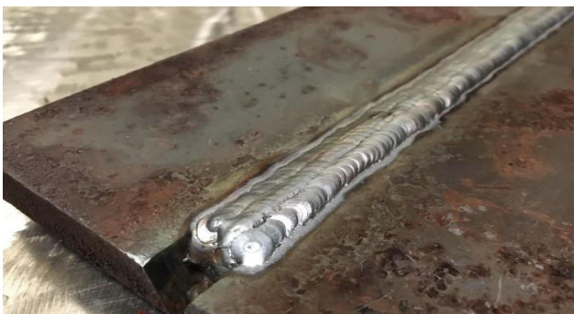
Figure-3. Open root "V" groove.
