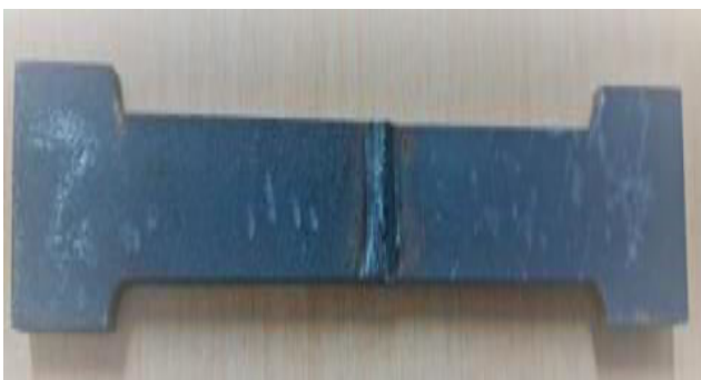
Figure-6. Sample for tensile test.
