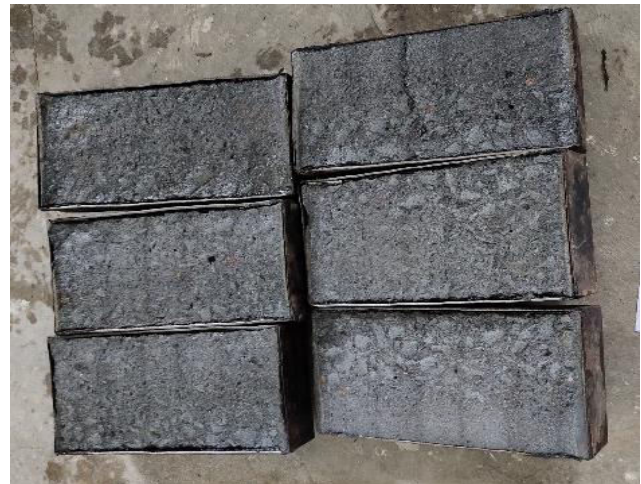
Figure-16. Concrete surface after 3 hours of abrasion testing.
