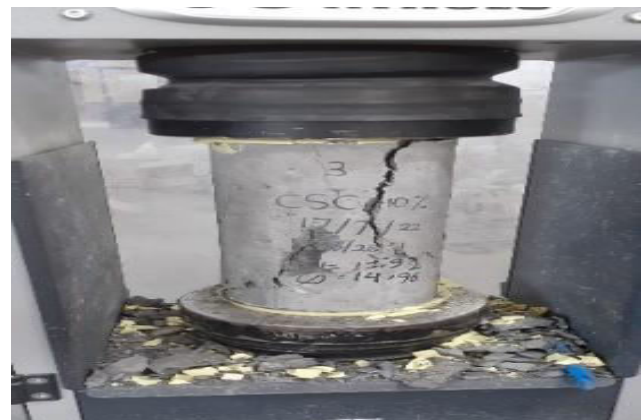
Figure-4. Compressive strength test.
