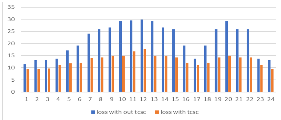
Figure-9. Generation losses between with and without TCSC.
