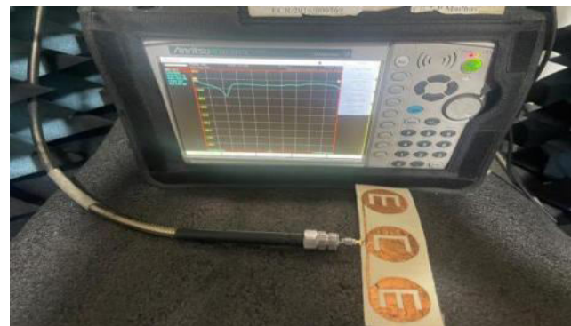
Figure-12. The antenna-4 proposed antenna S11 at free space.
