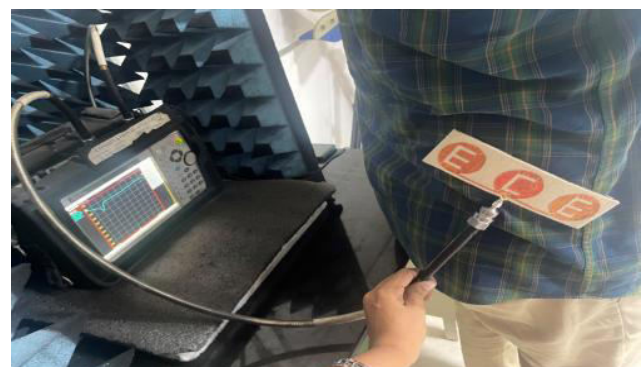
Figure-13. The antenna-4 proposed antenna S11 on the human body.
