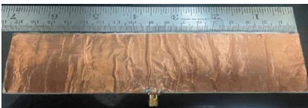
Figure-11. Bottom view of the proposed antenna-4 array.
