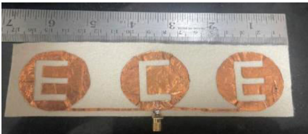
Figure-10. Top view of the proposed antenna-4 array.
