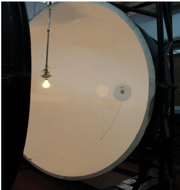
Figure-1. Integrating sphere to measure the flux.
