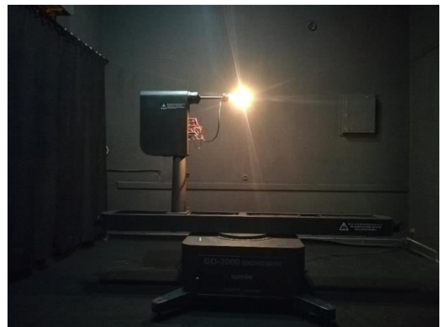
Figure-2. Goniophotometer to measure the luminaire flux.
