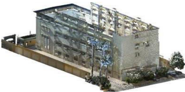
Figure-8. Engineering research institute and renewable energy 3D laser scanner survey 3D point cloud model.
