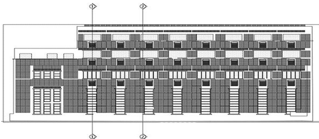
Figure-16. B: Alternative # 1 PVP panels elevation distribution.
