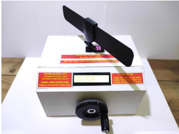
Figure-8. Tracking process of the antenna according to the set angle.
