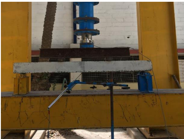
Figure-13. Beam 1-3 tested on loading frame.
