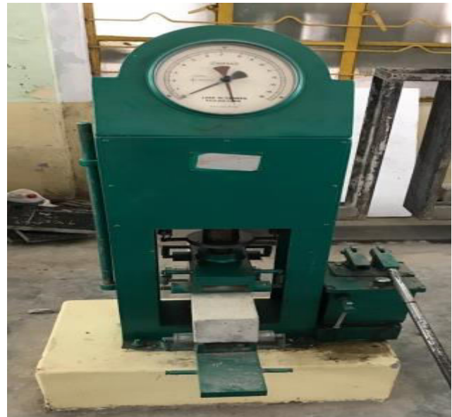
Figure-8. Bending strength of concrete prism.
