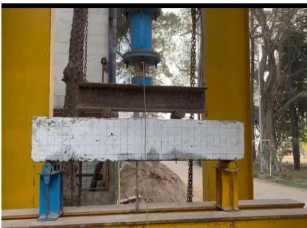
Figure-14. Beam 4-6 tested on loading frame.
