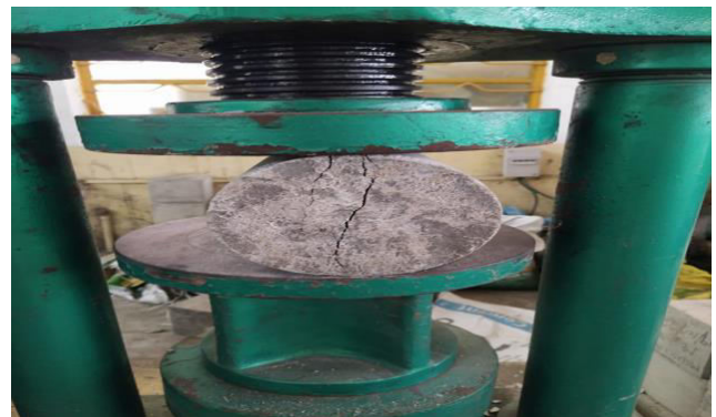
Figure-6. Splitting tensile strength of concrete cylinder.
