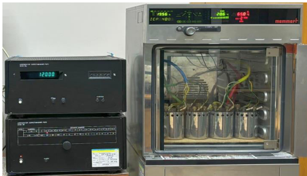
Figure-1. The general view of the precision measurement setup for the calibration of low-resistance measures.
