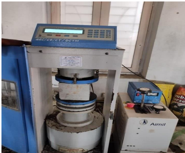
Figure-4. Compressive strength testing.
