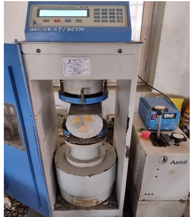
Figure-5. Split tensile strength testing.
