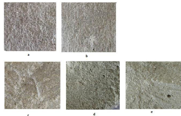
Figure-5. Macroscopic surface morphology of hardened cement paste specimens at 28 days of hydration (10× magnification): (a) Control sample (0% SCO), (b) 1% SCO. (c) 1.5% SCO (d) 2.5 % SCO (e) 5% SCO.
