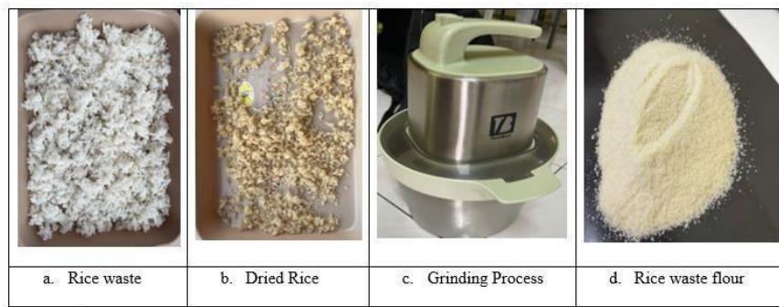
Figure-1. Rice waste powder step processes (a) Raw rice waste (b) Dried rice waste (c) Grinding process (d) Rice waste flour.
