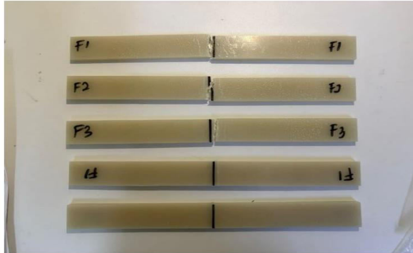
Figure-4. Sample of flexural testing.
