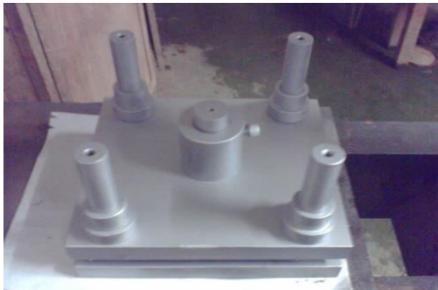
(a) Punch or the male part of the device
