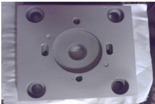
(b) Die the female part of the device
