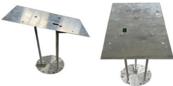
Figure-7. Component balance rig for experimental model.
