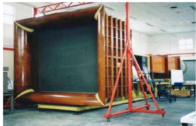
Figure-9. The Open Loop Wind Tunnel (Courtesy UPM-LST) with wind speed capacity is up to 50 \text{ ms}^{-1} [17][20].
