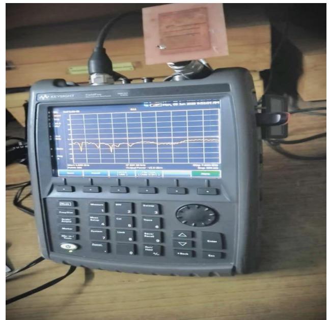
Figure-8. Experimental graph return loss vs. frequency using a spectrum analyser.
