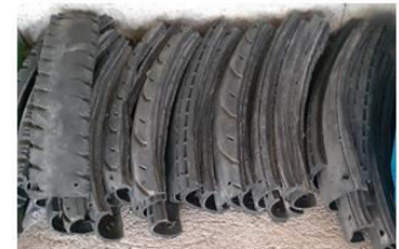
b) cutting of end-of-life motorcycle tires
