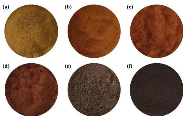
Figure-1. Images of Raw RG and Calcined RGs (CRGs) at different temperatures: (a) Raw RG, (b) 900°C CRG, (c) 1000°C CRG, (d) 1100°C CRG, (e) 1200°C CRG, (f) 1300°C CRG.
