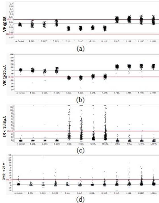
Figure-8. The electrical parameter and distribution for each of the cells from DOE. (a) The VF distributions for all the cells at 3A biasing testing. (b) The VR distributions for all the cells at 20  $\mu$ A biasing testing. (c) The IR leakage test distributions for all the cells at 3.48 A limit. (d) The Delta VR testing distribution for all the cells between two biasing, 20  $\mu$ A and 100  $\mu$ A.
