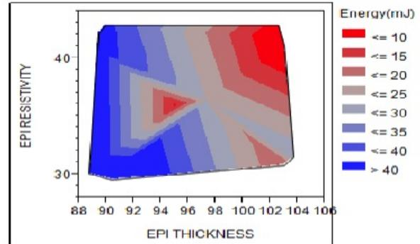
Figure-9. Contour plot for energy of UIS.
