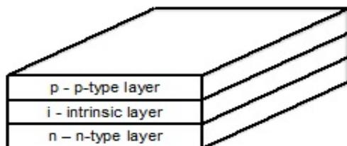
**Figure-1.** 2D structural layer P-i-N diode.
