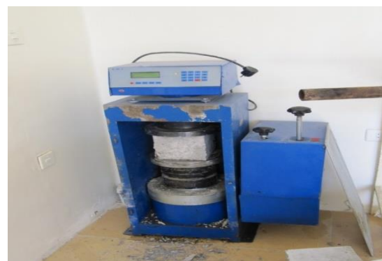
Figure-2. Apparatus for determining compressive strength of concrete RCC cube samples.
