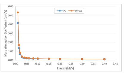
Figure-2. The mass attenuation coefficient of PC material compared with the human thyroid
